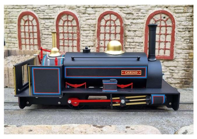
Other details include chimney, dome, safety valve bonnet, safety valve (attaches to rear of firebox and inserts into slot in safety valve bonnet).
