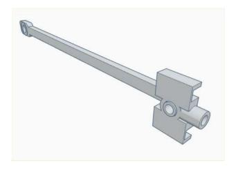
Place a washer over a crankpin, this washer will keep the rods off the cranks and stop them fouling as the wheels rotate. Now drop an ABS tube over the crankpin. The long ABS tubes for the rear crankpins, the shorter tubes for the front.
