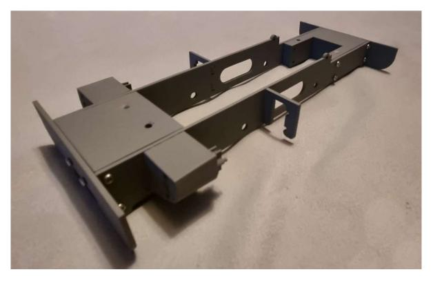
Note the motion brackets on each frameplate, and the correct orientation for the bracket, top & bottom. I painted the frame-plates once the brackets & cylinders were in place.
