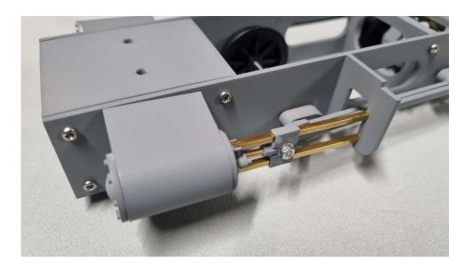
The rear cranks will also require the coupling rods fitting.
