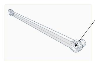
Create a better countersunk hole in the rear of the connecting rods, small end.
