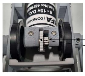
Locate the two gearbox parts. (Photo is VARSITY, but the gearbox is the same on CARIAD.).
