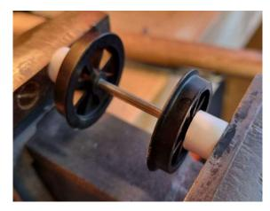
The second axle requires a brass top-hat bush be placed either side of the grey gear, between the wheel & grey gear. The lip of the brass top-hat bush must be flush against the grey gear on both sides. Again, use the white tube jig to ensure the wheels are pushed onto the axle to the correct depth.
