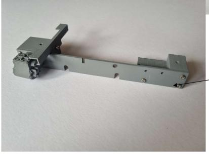
Now take the front & rear stretchers and using a further six M2 screws, attach the stretchers to the two stretchers to the frameplate. Now using six more M2 screws, attach the other frame-plate.
