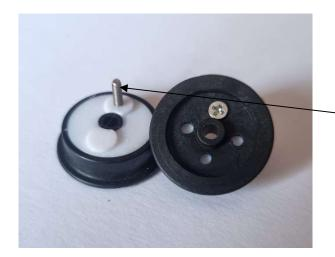
Squeeze the wheels onto the axles using a vice.
